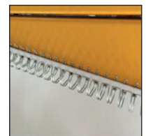
Getting through the hole with the suitable wire
